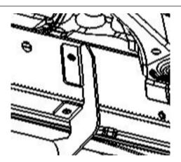
Step 4 After final adjustment tighten the lower mounts first then the upper mounts.
