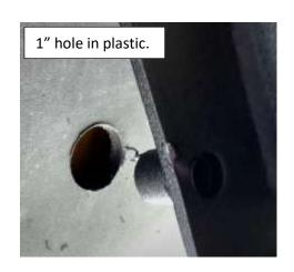
**Step 3**. Hold the bar up to the truck again, line up the holes you drilled, take 5/16 carriage bolt and insert through bracket and holes; install all 6 bolts with washers and hex nuts. Finger tighten so nerf step is suspended.
