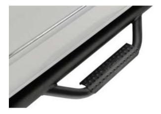
**Step 1.** To determine which is the front of the step, look for the shorter tail bend. Hold the N-Fab nerf-step up to the truck, approximately <sup>3</sup>/<sub>4</sub> to 1 inch from the front wheel well opening. (If you have oversized tires you can mount further back to ensure clearance.)
