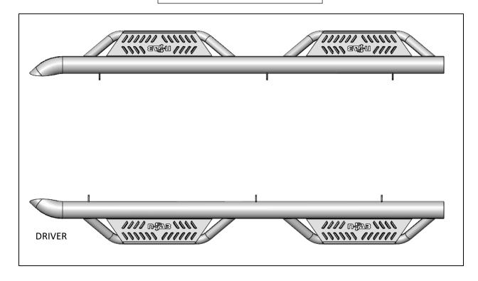
**Step 2.** Using the supplied M10 carriage bolt and nut, install the (x6) mounting brackets to each attachment point on the main tube and leave loose for now.
