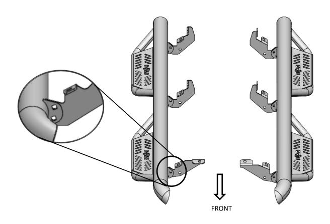
**Step 3.** Remove any factory running boards or hardware and discard. **Step 4.** Clean/tap the three factory threaded mounting locations.
