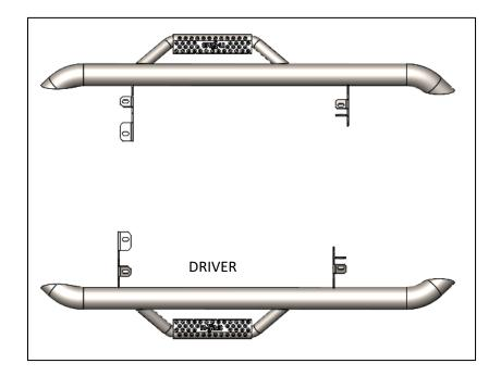
**STEP 2:** Remove any factory running boards or hardware and discard. **STEP 3:** Clean/tap the three factory threaded mounting locations.
