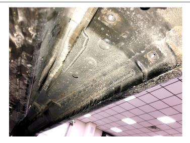
**STEP 4:** Carefully place step into place and loosely fasten using the supplied M10X25mm hardware.
