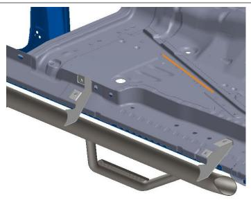
Step 5: Next, tighten the three lower bolts first following with the three upper bolts.Step 6: Repeat steps 2-5 with passenger side.Step7: Your install is now complete.
