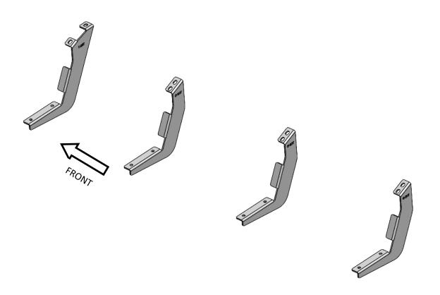
**Step 3:** Set running board along the top of all four brackets and center along the cab.
