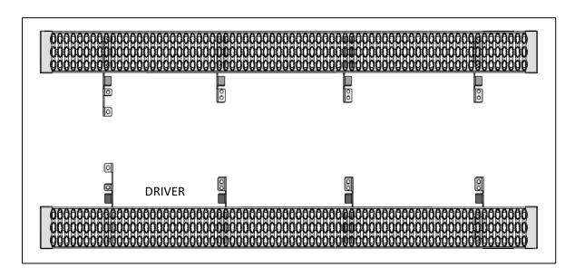
**Step 1** Beginning with the driver side, remove the factory hardware and discard. **Step 2** Next, install the (X4) rocker panel mounting brackets with the supplied M8x25mm Hex bolts with integrated washers and leave loose.
