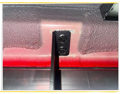
5. Next, adjust the step assembly up/down and front/back to level out the step rail with body panel and then tighten step to brackets at 20 ft. /lbs
