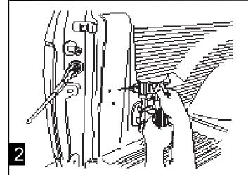
Using a power drill and 9/64" drill bit, drill through the sheet metal. If equipped with a bedliner, drill through bedliner.
