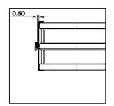
Note: The tube edge is approx .50" from the edge of the angle bracket.
