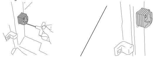
Proceed with Xtender instructions and adjust to the proper width. Install into angle brackets. Rotate Xtender inboard and outboard to verify tubes clear rails. If tubes do not clear add appropriate spacers. Reinstall tailights.
