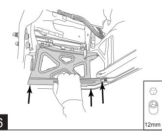
Replace Re enforcement bracket (15-03927-90). Reinstall bolts from step 6 and 7. Use provided nuts (19-03853-90) to secure bracket in place. Replace bumper components from steps 2-5.
