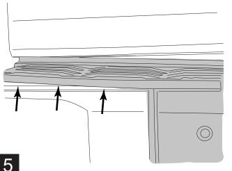
Lift bumper cap away and loosen and remove 2 upper bolts holding Re enforcement bracket in place.
