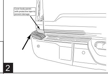
Remove license plate light by rotating and pulling out. Squeeze metal tabs holding trailer hitch plug and remove.
