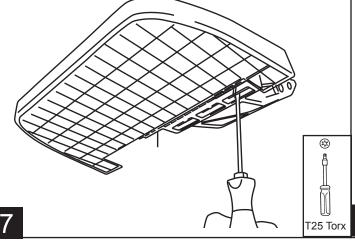
Torque bolt and two factory nuts from step 4 to 20 ft-lbs.
