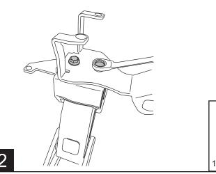
Drop threaded plate into slot in frame. Slot is located on both sides of the frame. The outer slot is preffered but may not be accessable with aftermarket bumpers or racks.
