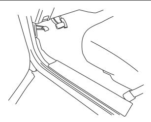
Open driver door and remove sill plate and kick panel.
