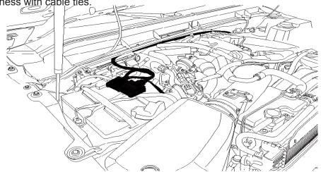
Run wire legs down and along underside of vehicle floor, securing with tie wraps. Run trigger wires (2) on Drivers side through grommet as shown bellow.
