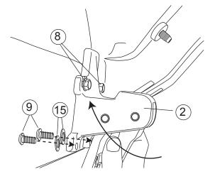
Note: Excursion requires hole to be drilled in body for rear linkage. Use 25/64" Drill Bit.
