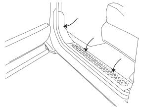
Plug in motors (both sides). Route remaining LED light wires back towards rear of vehicle.
