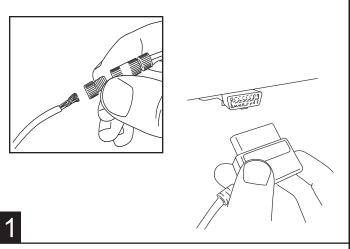
**OBD II install:** Use Supplied Posi Twist connectors to attach the Plug and Play Module to the Harness. Attach matching colors on the harness to the wires on the module. Plug in module to OBD II port on the vehicle. Secure harness with supplied tie wraps.
