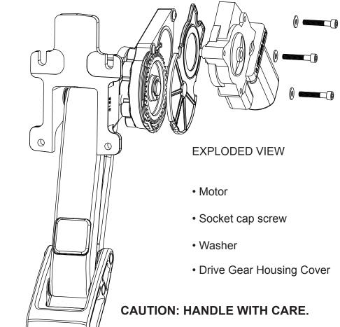
To ensure our customers receive all components with full integrity, we pack the motors separate from their linkage assemblies. This requires that the installer position and fasten the motor before continuing with the install. Please follow the instructions below and handle the assembly carefully.
