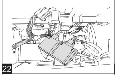
Route Trigger wires (Solid Purple and Purple / Black Stripe and module power wire) under seat and out under sill plate cover.
