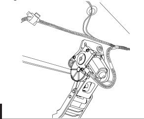
Connect red and black power leads to battery accessory studs. Red lead goes to positive. Route shorter leg of harness down passengerside wheel well and longer leg of harness down along driver side wheel well. Secure with tie wraps.
