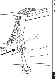
Close and wrap with conduit and electrical tape. Secure all loose wires with cable ties with lamp wires pulled upward to avoid any wire snagging.
