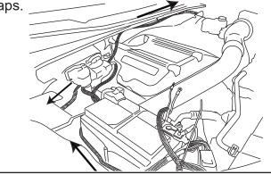
Remove driver side front kick panel and door sill plate. Roll back carpet to access hole for passing trigger wires into cab of vehicle.
