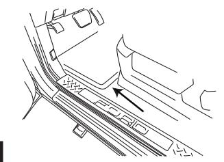
Remove grommet in floor panel above front linkage on driver side. Poke small hole into grommet and thread the two trigger wires through and up into the cabin of vehicle. Seal grommet with silicone sealer.
