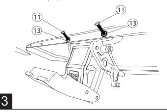
Mark the center of the forward most slot for the rivet nut hole. Once done then remove linkage.
