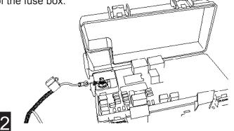
The two purple wires left from the harness will connect with wires that will be fed through from under the passenger side. See next steps.
