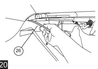
Pull down carpet on dash lower/center on the driver side and pull the tube through from passenger side. Note: When feeding tube thru, make sure to position it under existing wire harness (see picture) to keep the wires away from the silver AC/Heater tubing as that part may get hot and cause damage to wires. Once the tube is fed thru, feed both purple wires thru the tubing tool. The tube can now be pulled off.
