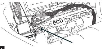
Route driver side leg down thru engine bay as seen here.
