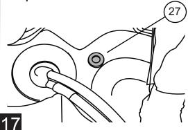
Use a lubricant on the two purple wires provided with the wire harness (7). Starting from the passenger lower compartment feed each wire thru the grommet up to the engine compartment. Make sure to feed one wire at a time, and pull wires careful to prevent grommet from coming out.
