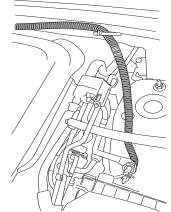
Open the Fuse box, (see step 10 for location of fuse box in engine compartment) connect the Red wire to positive power post located on top left corner of the fuse box.
