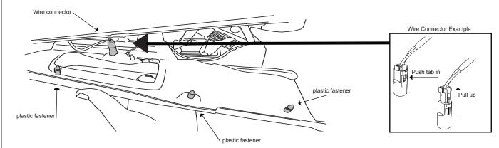
A. remove the three plastic fasteners with a soft pry tool.
