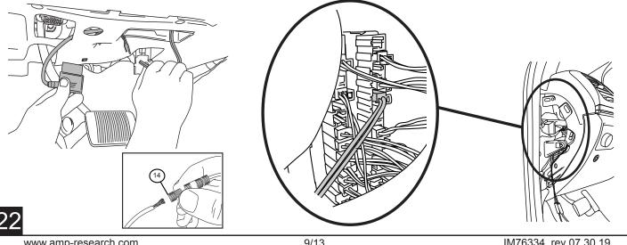
**OBD II install:** Use Supplied Posi Twist connectors to attach the Plug and Play Module to the Harness. Attach matching colors on the harness to the wires on the module. Plug in module to OBD II port on the vehicle. Secure harness with supplied tie wraps. *Note: If the OBD II pass thru harness (76404-01A) was purchased see install sheet supplied in packaging. The pass through harness allows for an open port for other accessories. See below for a brief description.*
