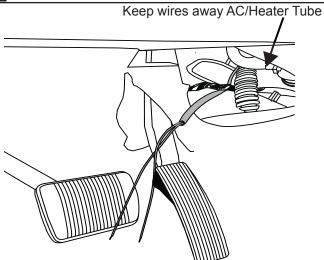
Feed wires thru the under dash cover as shown to keep wires tucked up out of the way. Connect the OBD Il plug to the trigger wires with Posi Lock Connector (14). Connect the matching wire color/stripe. Next, remove side access panel and connect 2 pin plug on OBD Harness into white bank of open ports as shown
