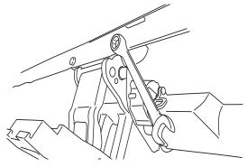
Install the Conical bolt in the installed Rivnut. Use spacer between linkage and rivet nut hole. Line up Conical Washer bolt (20) to Spacer (25) through slot, as shown below.
