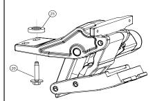
Note: If skid plate is present use shim (22) under skid plate, instead of spacer (25).
