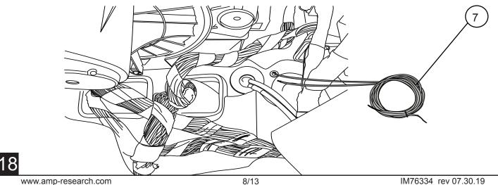
Connect the two purple wires coming from under the passenger side to the two wires in the engine compartment. Use Posi locks to connect them.
