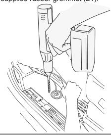
Route wire harness along the frame and back towards rear linkages. Secure with zip ties. Push both wires through rubber grommets.
