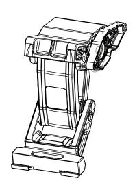
Motor Linkage assembly Passenger
