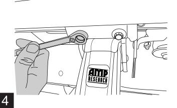
Install provided spacer (19) and M6 bolt (11) into upper mount as shown on both the drive and idler linkages. Do not tighten.
