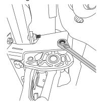
Attach motor to linkage. Using a 13mm wrench Torque to 36 in-lbs.
