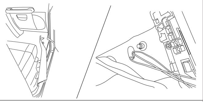
Mount door trigger module to wire harness in kick panel area. Using a 10mm socket remove ground lug and connect ground to body. Using supplied butt connectors connect red wire on harness to red wire (Pin1)on module. Next connect Purple with black stripe wire on harness to purple with black stripe from module (pin 6). Lastly connect Purple from harness to purple on module (Pin 7). See next step for trigger wire assembly.
