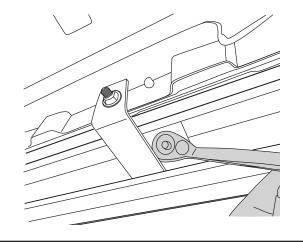
Mount front drive linkage onto driver side. Thread supplied bolts (15) into front drive linkage. Repeat step for Rear idler linkage. Do not tighten.
