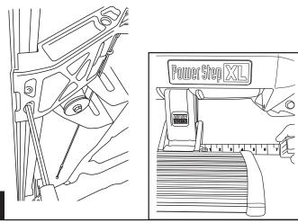
Using a 13mm socket Torque linkage bolts 4x (15) from step 3 to 16 ft-lbs. Next use a 10mm socket, torque linkage spacer bolt 2x (11) from step 6 to 8 ft-lbs. Once linkages are tight cycle board to verify steps deploy under own weight.
