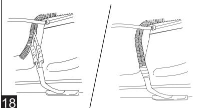
Reinstall Fuses from Powerstep Wire Harness.
