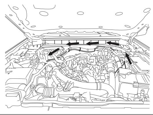
Locate oval grommet on driver side of firewall and push out. Poke small hole in grommet and thread trigger wires into cab of vehicle.
