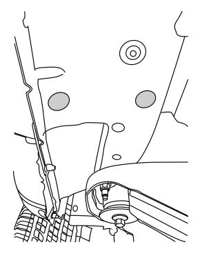
Attach bracket (27) using M10 Hex Flange Bolts (8).
