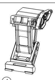
Motor Linkage assembly Passenger
