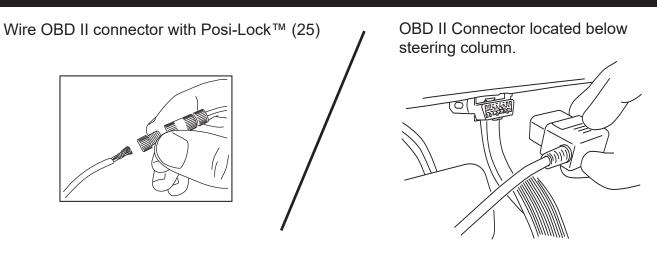
**OBD II install:** Use Supplied Posi-Lock<sup>™</sup> (25) connectors to attach the Plug and Play Module to the Harness. Attach matching colors on the harness to the wires on the module. Plug in module to OBD II port on the vehicle. Secure harness with supplied tie wraps. *Note: If the OBD II pass thru harness (76404-01A) was purchased see install sheet supplied in packaging. The pass through harness allows for an open port for other accessories. See below for a brief description.*
