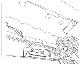
Using supplied butt connectors (19), connect the lamp wires. Red to Red, Black to Black. Once Crimped use heat gun to shrink tube. Close and wrap conduit with electrical tape. Secure all loose wires with zip ties (16). Pull lamp wires upward to avoid any wire snagging.
