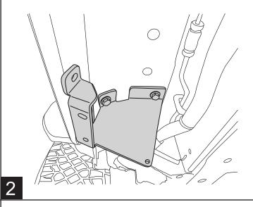
Locate **Rear Drive linkage** location. If plastic plugs are present remove plastic plugs to expose threads.
