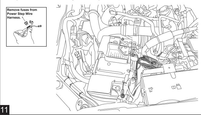
Route the two wire harness legs down over to each wheel well. Long leg will run across to passenger side, short leg will run down to driver side. Ensure loom is free from steering and exhaust components. Secure harness with Zip Ties (16).
