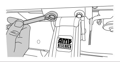
Install provided Spacer (15) and M6 Bolt (10) into upper mount as shown on both the Drive and Idler linkages. Do not tighten.
