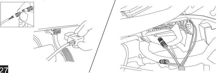
Secure harness with supplied tie wraps. Make sure wires are away from E-brake mechanism and brake pedal assembly.
