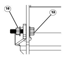
Attach motor to linkage. Using a 4mm hex Torque to 36 in-Lbs.
