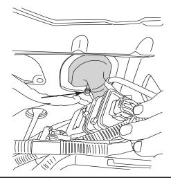
Tape leading end of wires together and push through rubber boot to cabin side of the firewall. Silicon lubricant may be used for ease of passage. The trigger wires will come out just above and to the left of the brake pedal.
