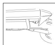
Using a 13mm socket Torque linkage bolts 4x (9) from step 3 to 16 ft-lbs. Next use a 10mm socket, torque linkage spacer bolt 2x (13) from step 6 to 8 ft-lbs. Once linkages are tight cycle board to verify steps deploy under own weight.
