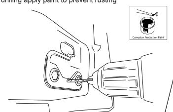
Once hole is drilled insert a piece of string or wire through hole in Reinforcement Plate. Set plate into position.
