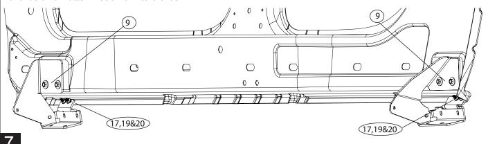
Insert and position Carriage bolts (16) into slot on rail (4). Insert from either end of rail. Using Flange Nuts (17) provided assemble rail to Brackets onto the rail. Next install Flange Bolt (14) and Flange Nut (10) onto bracket tab. Driver side shown. Dimensions shown are for reference. *Torque flange nuts to 16ft-lbs.*
