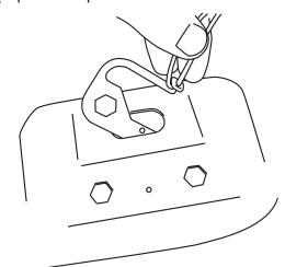
Set rivet nuts into place for alignment. Insert pop rivet through hole in plate and secure in place. Once pop rivet is installed remove string or wire from Reinforcement Plate. **NOTE: Verify plate is pulled flush to the body before securing pop rivet.**
