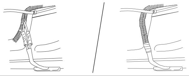
**OBD II install:** Use Supplied Posi Twist connectors to attach the Plug and Play Module to the Harness. Attach matching colors on the harness to the wires on the module. Plug in module to OBD II port on the vehicle. Secure harness with supplied tie wraps.
