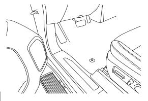
Route wire harness along the frame and back towards rear linkages. Secure with zip ties. Push both wires through rubber grommets.
