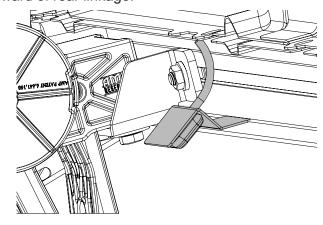
Using supplied butt connectors(23), connect the lamp wires. Red to Red, Black to Black. Once Crimped use heat gun to shrink tube. Close and wrap conduit with electrical tape. Secure all loose wires with cable ties. Pull lamp wires upward to avoid any wire snagging.
