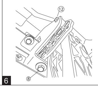
Verify rail clearance at front fender trim and push upwards on rail to ensure rail is snug to the bottom of the linkage mounting bracket. Using a 1/2" socket start at the rear of vehicle and work forward. Torque 5 flange nuts (15) to 16ft-lbs. Tighten mounting bracket hardware from step 1. Torque to 16ft-lbs
