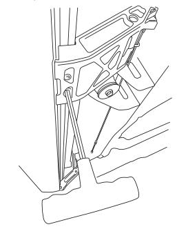
Using a 13mm socket Torque linkage bolts 4x (9) from step 5 to 16 ft-lbs Next use a 10mm socket, torque linkage spacer bolt 2x (12) from step 6 to 8 ft-lbs.
