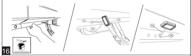
Using supplied butt connectors (13) connect the lamp wires. Red to Red, Black to Black. Once Crimped use heat gun to shrink tube. Close and wrap conduit with electrical tape. Secure all loose wires with cable ties. Pull lamp wires upward to avoid any wire snagging.
