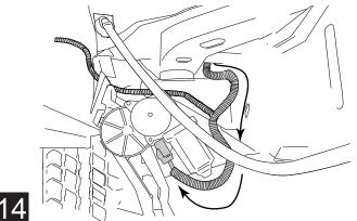
On Passenger Side, run Wire Harness leg down and along underside of the vehicle floor and frame to front Drive Linkage. Connect harness to motor and secure harness with tie wraps. Route remainder of wire harness towards rear linkage assembly for LED lights
