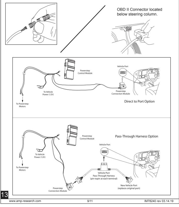
On driver side, run Wire Harness leg down and along underside of the vehicle floor and frame to front Drive Linkage. Connect harness to motor and secure harness with tie wraps. Route remainder of wire harness towards rear linkage assembly for LED lights
