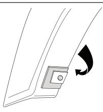
WRAP BLACK MYLAR TAB OVER HOLE, THEN INSTALL S-CLIP ON TOP OF IT.
