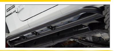
Step 6. First, tighten all hardware that attaches the bracket to the pinch weld of the vehicle. (15-20 ft/lbs)
