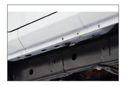
Step 2. Carefully raise up (#1) driver side rail into position and align the brackets with the factory mounting points with the horizontal part of the bracket on the outside of the pinch weld.
