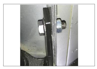
Step 7. Next, tighten the remaining hardware that attaches the bracket to the upper body mount. (15-20 ft/lbs)
