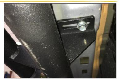
Step 4. Start two (#4) M8x25mm black zinc flanged bolts and two (#5) M8 flanged nuts (both brackets) in the pinch weld and leave loose for finial adjustment.
