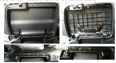
On either end of the hinge is a plastic cover that must be removed next. You can use a small screw driver or even a finger nail. Detailed photos on back.
