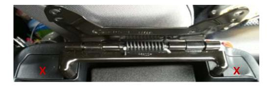
Red X's mark plastic covers that must be removed tp access hinge screws.
