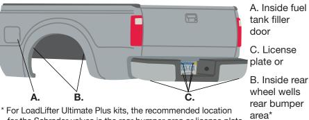
\* For LoadLifter Ultimate Plus kits, the recommended location for the Schrader valves is the rear bumper area or license plate.
