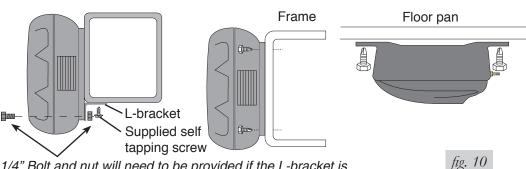
1/4" Bolt and nut will need to be provided if the L-bracket is fabricated. The L bracket is shown as an optional mounting method and is not supplied.
