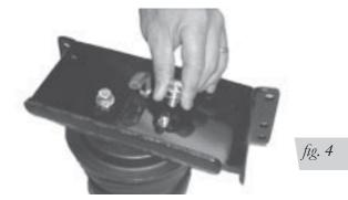
4. Attach the lower bracket (C) to the air spring (A) with flat washers (M), lock washers (N), and <sup>3</sup>/<sub>8</sub> x <sup>7</sup>/<sub>8</sub>" hex head bolts (L). Refer to Figure 5. Tighten to 20 ft-lbs.
