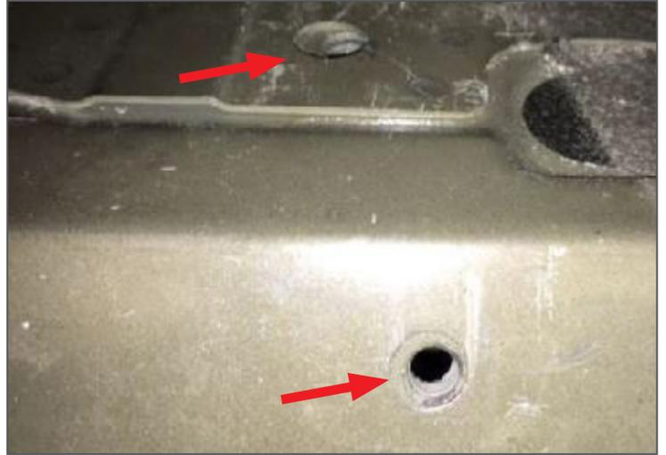
Step 2. Next, start x3 (#3) M8X30mm Hex Cap bolts in the upper mounts only and leave loose. **NOTE: Make sure you only engage enough threads so the bolt can easily slide through the upper mount attachment point.**
