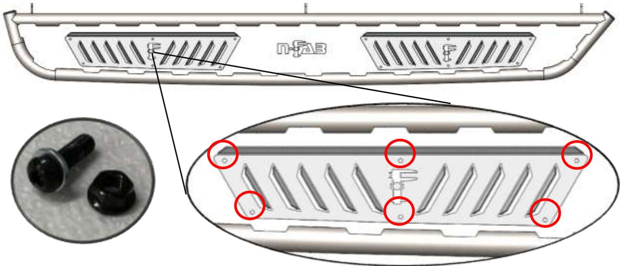
**Step 3:** Install the supplied rocker panel brackets (x6) to the attachment points located on the backside of the main tube (Driver/Passg) using the supplied 3/8" x 1" carriage bolts and 3/8" flanged nuts. Leave finger tight for now.
