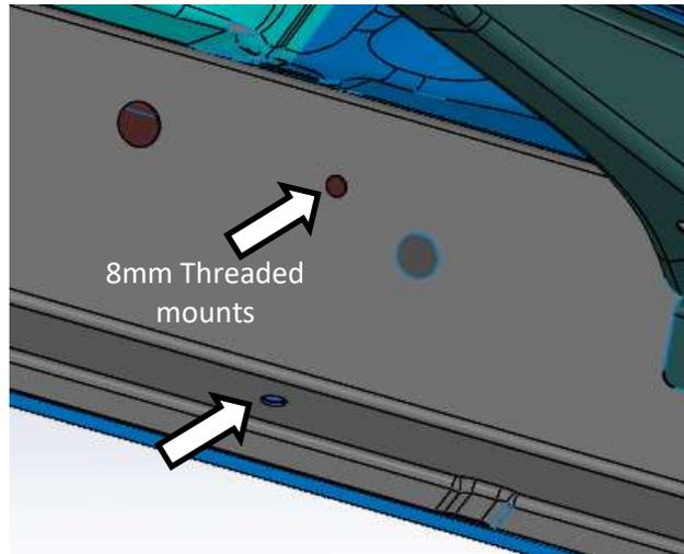
**Step 5:** Carefully raise the Nerf Board assembly up into position aligning the mounting brackets with the factory-threaded holes. Beginning with the center bracket start one of the supplied M8x30mm Hex bolts in the upper mount and finger tighten. This will allow the step to suspend while you start the remainder of the hardware.
