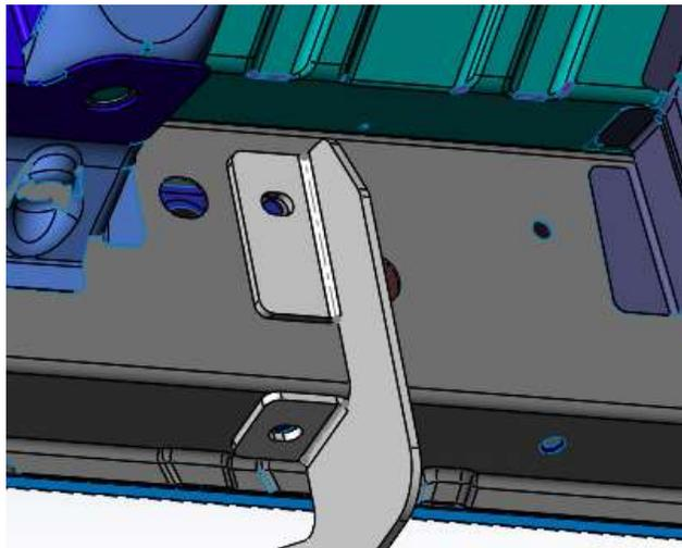
**Step 8:** There will be  $\frac{1}{2}$ " of adjustment in the (x3) mounting bracket. Adjust to desired position and tighten to (20 ft./lbs).
