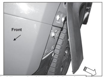
(Fig 4) Use panel tool (not included) to release plastic clips. Carefully pull fender flare straight out to access (4) screws attaching bumper cover to fender.
