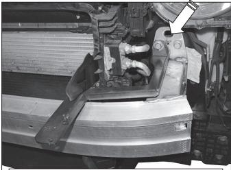
(Fig 9) Reuse factory hex bolt (arrow) to attach driver/left Top Bracket to bumper bracket
