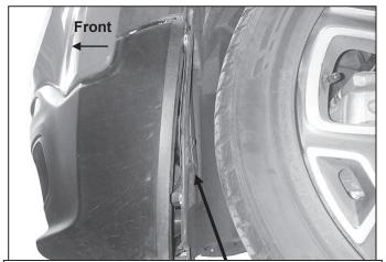
(Fig 3) Remove hardware attaching fender to fender liner. Pull back liner to access and unplug lights
