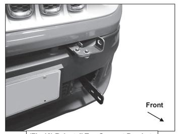
(Fig 18) Reinstall Top Support Brackets
