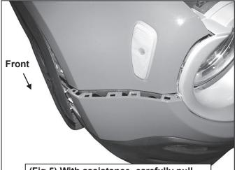
(Fig 5) With assistance, carefully pull bumper cover and grille assembly off of vehicle (passenger/right side pictured)
