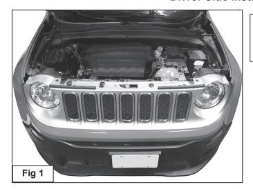
Remove hardware attaching the top of the grille to the radiator core support. Remove the hardware attaching the bottom of the bumper cover to the bottom of the radiator core support.
