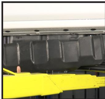
**STEP 8** (Passenger Side): First bracket has a tab that locates in the OE body mount hole.
