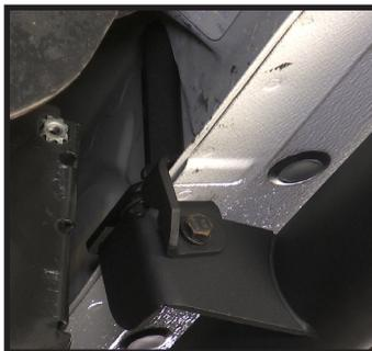
**STEP 13** (Passenger Side): Use 13mm bolt to align 2 piece bracket to the board, insert at the side and hand tighten. Apply to both first and second bracket.
