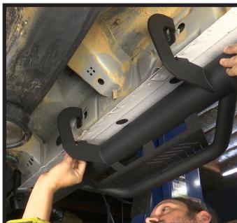
**STEP 12** (Passenger Side): Carefully place passenger side step into place. Use bolt, washer and begin hand tightening both upper mountings and pinch weld mounting to the rear two brackets. Best to have an assistant to lift and hold board in place.
