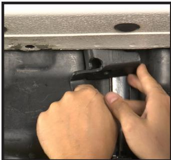
**STEP 10** (Passenger Side): The second bracket attaches to the body with a bolt rather than the tab like the first bracket.
