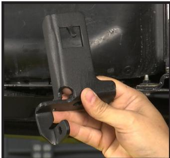
**STEP 9** (Passenger Side): Take bracket and feed between the body and the DEF tank, feel and move until you locate the tab into the OE hole. The bracket will hang once placed correctly.
