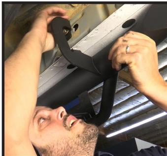
**STEP 16** (Passenger Side): **Avoid using power or air tools.** Tighten pinch weld mounts first then upper bolts. Tighten all hardware to 20ft lbs torque to secure the board to the truck.
