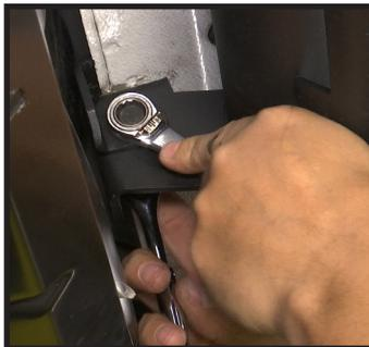
**STEP 15** (Passenger Side): Snug hardware for the first and second bracket. Tighten the bolt going up through the pinch weld first to pull the board into place. Then tightening both side bolts.
