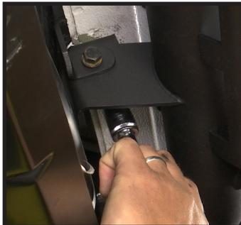
**STEP 14** (Passenger Side): Insert bolt and washer going up through board, truck pinch weld and through the 2 piece bracket.
