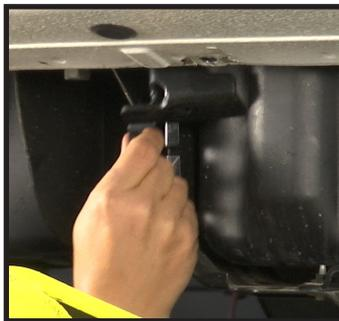
**STEP 11** (Passenger Side): Take bracket and feed between the body and the DEF tank from the back of the tank. You'll be able to fit and hand tighten bolt through the bracket to the body.
