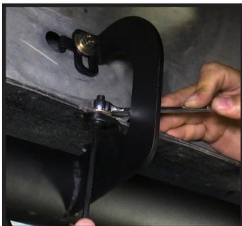
**STEP 7** (Passenger Side): Remove plastic shield from DEF tank on passenger side of the truck.
