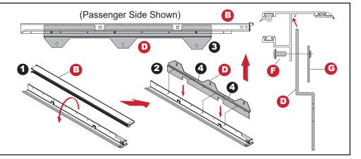
(1) Turn lock to 10 o'clock. (Do not remove plastic wing nut). (2) Align tracks (B) onto housing stem. (3) Make sure the edge of the tracks butt up against housing on driver and passenger side.
