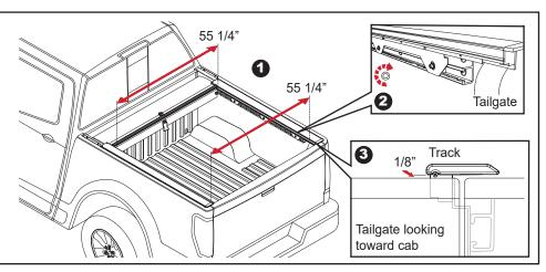
Turn lock to 7 o'clock (1), remove plastic wing nut (2) and using both hands pull cover back to tailgate.
