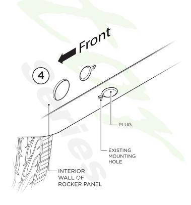
**5.** Remove the (2) plastic plugs from all (3) mounting locations in the rocker panel. Front Center and Rear. Insert M8 U Nut Clips so that the threads are on the inside of the rocker panel.
