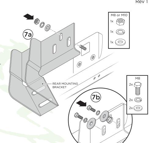
8a. If installing Rear Mounting Bracket **WITH** Rear Support Brace, position Rear Support Brace over the Rear Mounting Bracket and attach the top mounting point to the vehicle using M8 or M10 hardware depending on bolt plate used. You will use one (1) Flat Washer, one (1) Lock Washer and one (1) Hex Head Nut.
