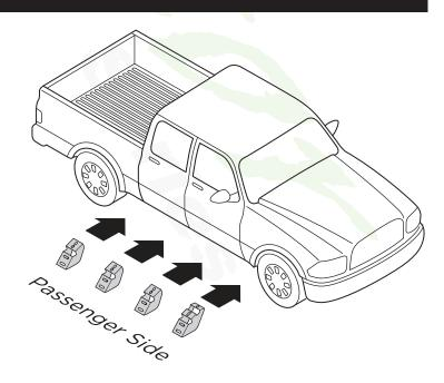
**4.** Align brackets with existing factory threaded holes in the rocker panel (4a). These holes may have black plugs in them that will need to be removed before installation. Fasten each bracket to the rocker panel using two (2) M8 x 30mm Hex Head Bolts, two (2) M8 Lock Washers and two (2) M8 Flat Washers (4b) per bracket.
