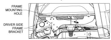
Figure C4: View looking into driver side wheel well.
