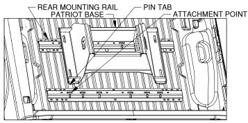
Figure E3: View into truck bed looking back at tailgate.
