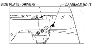
Figure D1: View looking into driver side wheel well.
