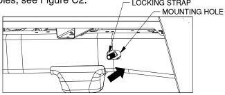
Figure C2: View looking into driver side wheel well.
