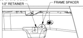
Figure C3: View looking into driver side wheel well.
