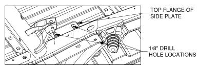
Figure C5: View under bed looking up at drilled area and side plate.
