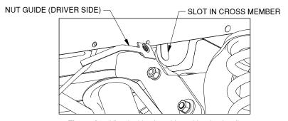
Figure G2: View looking into driver side wheel well.
