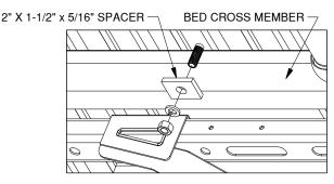
Figure D2: View looking up under the truck bed.
