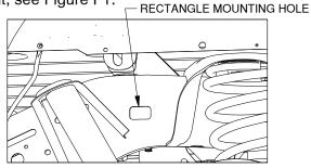
Figure F1: View looking into driver side wheel well.
