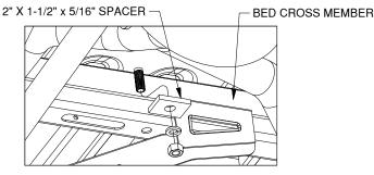
Figure D5: View looking up under the truck bed.
