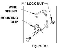
Figure D1: Leveling kit parts.
