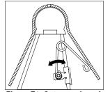
Figure F1: Cutaway view of driver side pivot arm and saddle.
