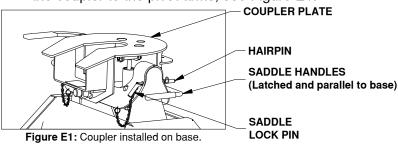
Set coupler angle. Adjust the resting angle of your coupler plate by rotating the spring on the driver side pivot arm. Pulling the top of the spring away from the cab will increase the angle of the coupler plate. Set the angle of the coupler so that head will tilt away from the cab when coupling, see Figure E2. Tighten the 1/4" nut once the springs orientation is set.
