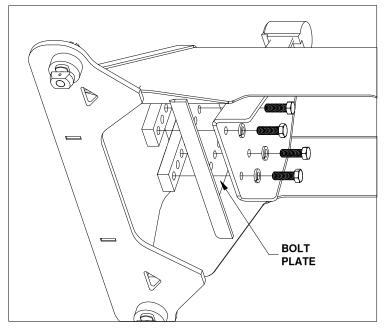
Figure A2: Passenger pivot arm mounting location.
