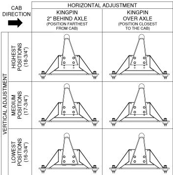
▲ WARNING: B&W recommends that you check the clearance between the truck cab and the trailer. Compare the measurement taken from the center of the Coupler to the cab, to the measurement taken from the center of the king pin to the farthest forward corner point of the trailer. These measurements will allow you to see how much clearance you will have between the cab and the trailer while towing and turning.
