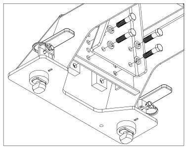
Figure A2: Passenger pivot arm mounting location.
