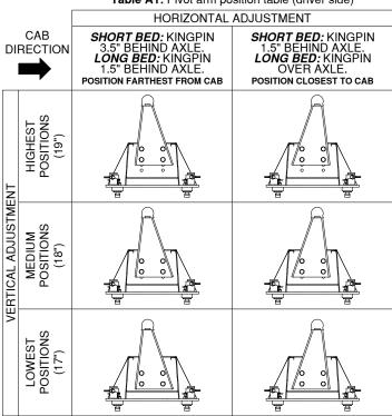
WARNING: B&W recommends that you check the clearance between the truck cab and the trailer. Compare the measurement taken from the center of the Coupler to the cab, to the measurement taken from the center of the king pin to the farthest forward corner point of the trailer. These measurements will allow you to see how much clearance you will have between the cab and the trailer while towing and turning.
