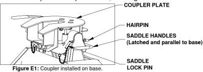
2. Set coupler angle. Adjust the resting angle of your coupler plate by rotating the spring on the driver side pivot arm.
