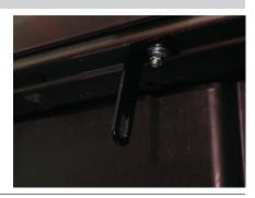
Slide an 8mm clip nut onto the mounting tab. Fasten the side bar mounting bracket with an 8mm hex bolt, flat washer and lock washer.
