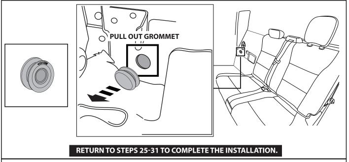
**35.** Locate the rubber grommet in the back of the back of the cab and push it out between the cab and the bed. Retain this as it will be re-inserted in step 28. Return to steps 25-31 to complete the installation.
