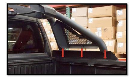
**STEP 9**: Mark any three holes along mounting bracket (per side) to attach sport bar, making sure the underside of the bed rail is free from any obstructions if possible. Some vehicles have perforations in the steel part of the bed rail. With caution, you may remove the plastic bed rail cover to verify where you are drilling is metal. Once this is determined, reinstall the plastic bed rail cover. Repeat steps for both sides. Remove Sport Bar once desired fit it achieved.
