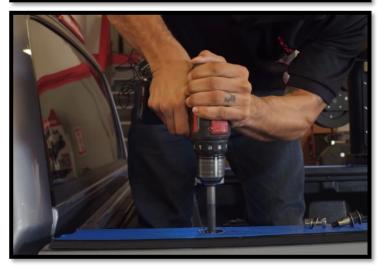
**STEP 10**: Use a 1/8" or 1/4" drill bit to make a pilot hole.
