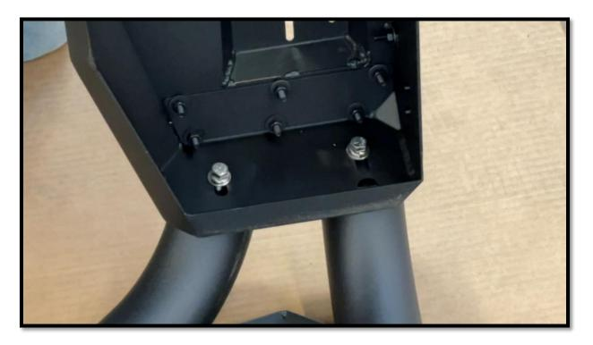
**STEP 5**: With assistance, install box assembly onto front and rear tubes as shown. Position the rear upper vinyl washer (item 14) and front top vinyl (item 13) in between the tubes and base plate. Fasten down using 3/8" hex bolts (2), 3/8" flat washer (2) and 3/8" lock washer (2). Leave finger tight for later adjustment. Repeat steps for passenger side.
