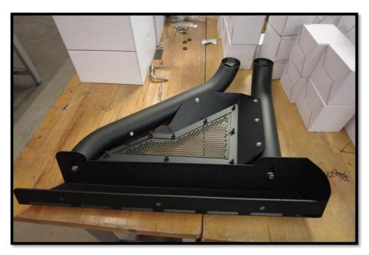
**STEP 4**: Install base plate onto front and rear tubes as shown. Position the rear bottom vinyl washer (item 16) and front bottom vinyl (item 15) in between the tubes and base plate. Fasten down using 3/8" hex bolts (2), 3/8" flat washer (2) and 3/8" lock washer (2). If you're planning on not using a tonneau cover with your Sport Bar, install the base plate cover on the bottom of the rear tube. Leave finger tight for later adjustment. Repeat steps for passenger side.
