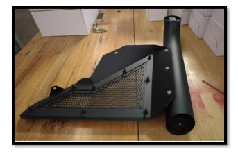
**STEP 2:** Attach front driver side tube (short) to the driver side mesh using ¼" button head screw (3), ¼" lock washer (3) and ¼" flat washer (3). Leave had tight for later adjustment
