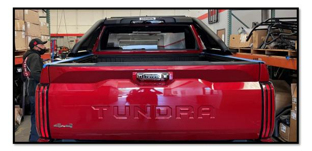
**STEP 7**: With assistance, position the Sport Bar 2.0 on the bed rails. Use painters tape to protect the OEM plastic. Begin to adjust the Sport Bar to your desired fit by moving the base plates , tubes and center box. Be sure that the vinyl spacers stay with the tubes to prevent metal to metal contact and preserve the life of the finish.
