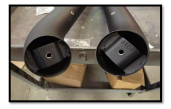
**STEP 1**: Identify driver side tubes. You can locate the D (Driver) or P (Passenger) stamping on the bottom of the tubes. The shorter tubes are the front tubes, the longer tubes are the rear tubes.
