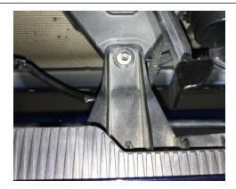
**Step 3** Next, remove the (x3) bolts that attach the inner fender (both sides). **Step 4** Remove the bottom (x2) bolts that attach the lower valance.
