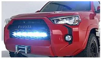
**Step 1** You will have to remove the front bumper. To do this, first remove the (x13) pushpins to release the plastic cover and remove.
