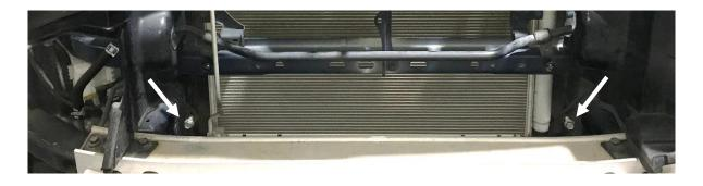
**Step 10** Install the passenger and driver side LED bracket. To do this, start with the lower mounting position using the factory M10 bolt removed in step 9. Leave loose for now.
