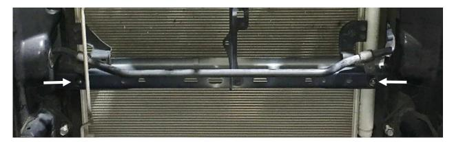
**Step 9** Remove the (x2) factory core support bolts and set aside, do not discard.
