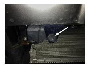
**Step 5** Remove the (x2) bolts from under the corner of the bumper (both sides).
