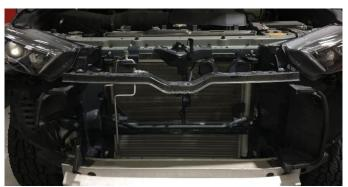
**Step 8** Remove the (x2) 6mm bolts that attach the cooling line to the core support and discard.
