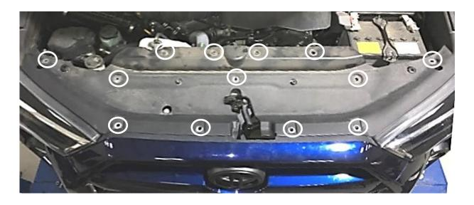
**Step 2** Remove the (x3) bolts that attaches the top of the grill. The will be one in the center and one to the left and right of the upper grill.
