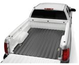
Place UnderLiner™ in the bed of your truck. Align contours and cutouts for the wheel wells to allow UnderLiner™ to lay flat and smooth.
