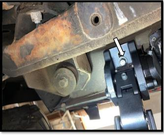
**Step 8**: . Install front passenger side bracket onto weld seam using (2) M8x20MM Hex Bolts, M8 Lock Washer, M8 Flat Washer. On the underside of the bracket, secure it to the motor to the mounting plate using (1) M8x35MM Hex Bolts, M8 Lock Washer, M8 Flat Washer.
