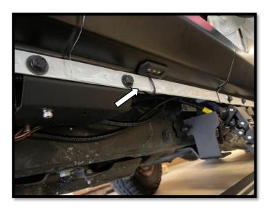
**Step 16**: Align the arrows on the small round connectors and plug the Passenger side front and Passenger side rear LED lights. Prepare the surface by cleaning with a 50/50 mix of isopropyl alcohol and water or equivalent. Once the surface is completely dry, peel the backing from the double-sided tape and stick the LEDs to the bottom side of the rocker panel. Position the LED lights at the center of the front and rear passenger side doors
