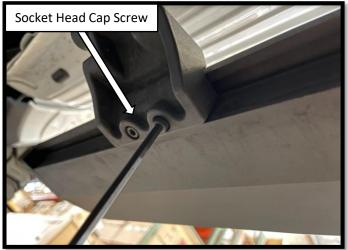
**Step 13**: Determine where you want to position the board and secure the running board to the arms using the (2 per bracket) M6x25 socket head cap screws. Using a torque wrench, tighten to 9 ftlbs. Step # With the running board is installed, fasten the hardware on the Passenger side front and rear motor assemblies. Using a torque wrench, tighten the mounting hardware to 18 ftlbs.
