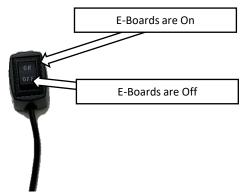
**Step 28:** Open the Driver side door and keep the door open. Flip the disable switch to the Off position. This will signal the running boards to retract to the stowed position and it will disable any further operation until the switch is flipped to the On position.
