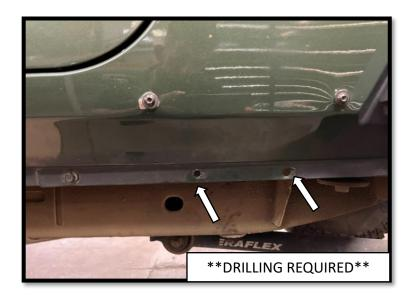
**Step 7**: Using a 21/64" drill bit, chase the two front motor mounting holes on the pinch seam. Use touch up paint to cover up any raw metal on the pinch seam.
