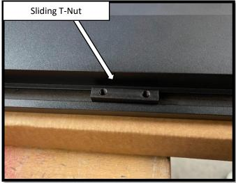
**Step 12**: Install the Passenger side running board. With assistance, begin by positioning the board on the front and rear motor assembly bases. Align the sliding T-Nut on the running board with the slots on the front and rear motor base. Once the T-Nuts are aligned, rotate the running board so that the T-Nuts set in the slots on the base of the arms. Repeat 1-11 to install the motor linkage assemblies and running board on the driver side side.
