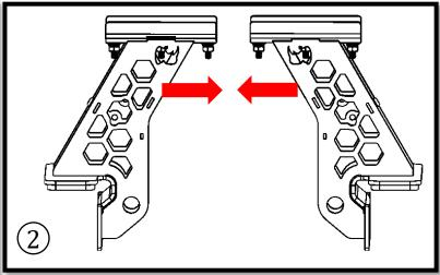
Install foam adhesive on the mounting surface of the SRM tower(image 1). Position each tower mounted be sure the Rhino heads are facing each other (image 2).
