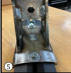
Install tower into crossbar with the ¼" exposed as studs (image 4). Secure each tower with 3 QTY with ¼" flat washer, ¼" lock washer, ¼" hex nut (image 5). Leave loose for final adjustment. Repeat steps for all four corners.
