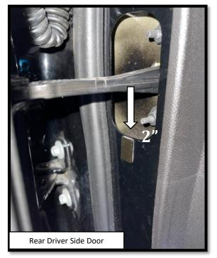
**Step 20:** With the rear driver side sensor attached, you can determine the correct position for the door magnet. peel the backing from the double-sided tape and stick the magnet on the door. Align the bottom of the magnet with the 4 1/2"
