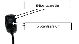
**Step 24:** Open the Driver side door and keep the door open. Flip the disable switch to the Off position. This will signal the running boards to retract to the stowed position and it will disable any further operation until the switch is flipped to the On position.
