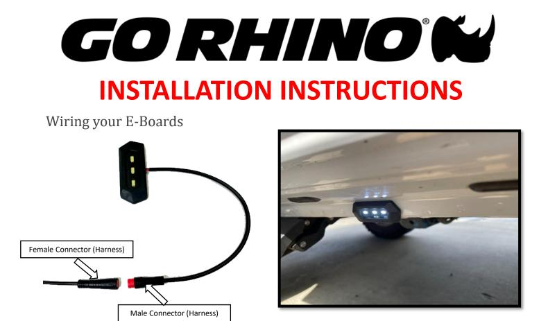
**Step 12**: Align the arrows on the small round connectors and plug the Passenger side front and Passenger side rear LED lights. Prepare the surface by cleaning with a 50/50 mix of isopropyl alcohol and water or equivalent. Once the surface is completely dry, peel the backing from the double-sided tape and stick the LEDs to the bottom side of the rocker panel. Position the LED lights at the center of the front and rear passenger side doors
