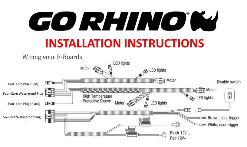
**Step 11:** Route the electrical harness from the controller along the frame rail of the truck. Connect the male plug connector on the wire harness into the female socket on the motors. The harness is labeled to show where to plug each male connector to the female connector. For example, Front Left is for the front Driver side motor and Rear Left for the rear Driver side motor. Use supplied zipties to secure harness to the frame rail.
