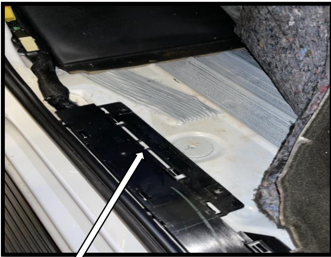
Passenger Side carpet, pull back to expose grommet opening
