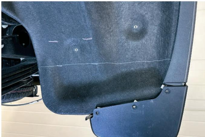
16. Cut the liner along the horizontal line made.
