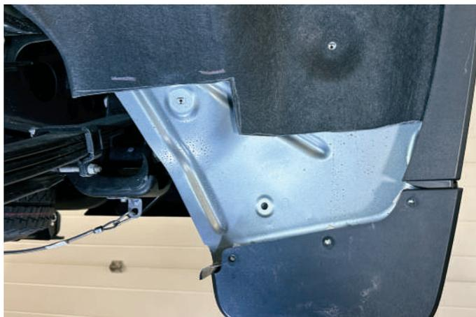
21. By trying to install the bracket, you can see where further relief is needed.
