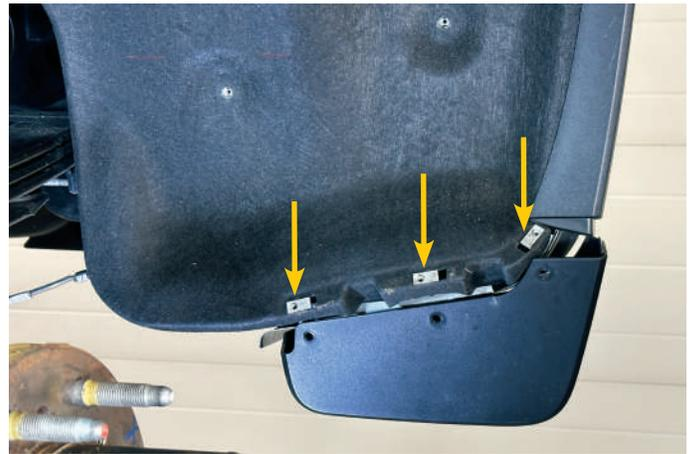
3. Remove the spring nuts from the liner.
