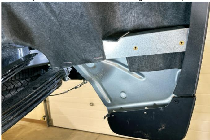
26. Reinstall factory screws as shown here.
