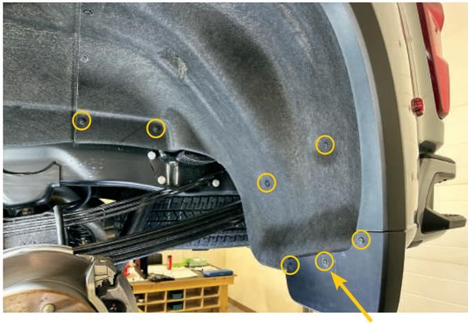
2. Pull the factory protector down so the spring nuts on the liner are exposed.
