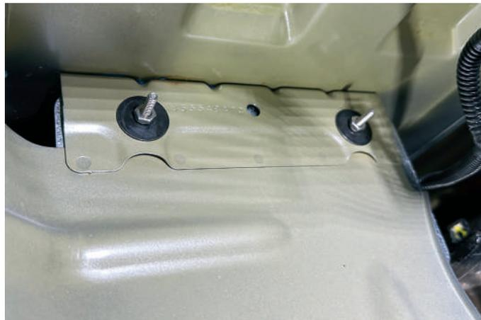
25. The bracket should now be installed & look like this. Ensure outer part of bracket is installed behind the wheel lip.
