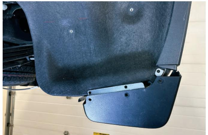
5. Reinstall spring nuts on the sheet metal as shown.
