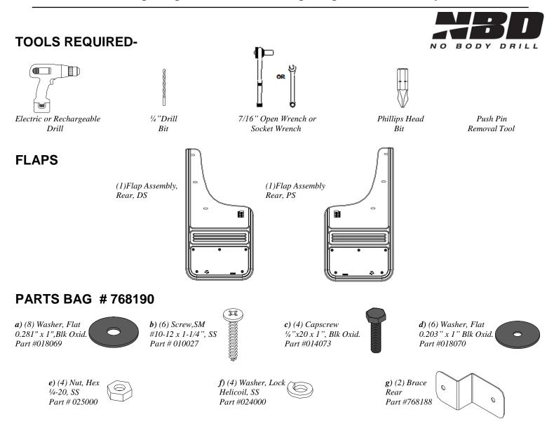
**INSTALLATION** (For ease of installation it is suggested that the wheel be removed)
